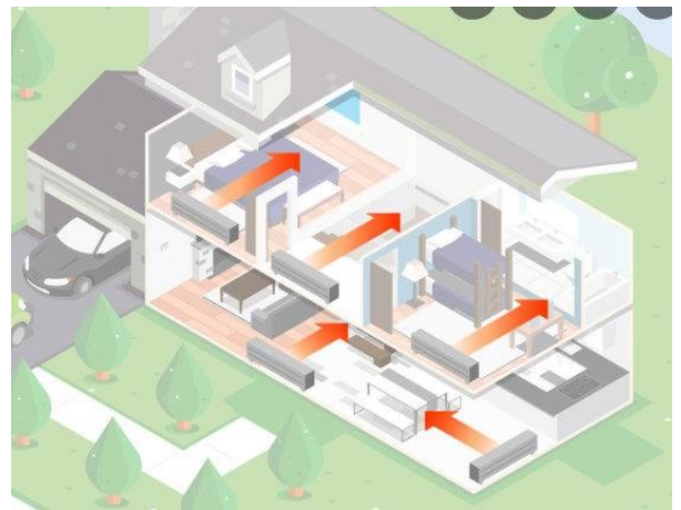
A typical electric baseboard heater that would be located in each room of a house
